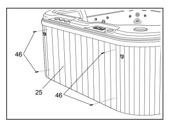
To replace the Access Panel, hold the Access Panel in place and secure it with the four  $#10 \times 2$ " Machine Screws (46). Be careful not to overtighten the Screws.
